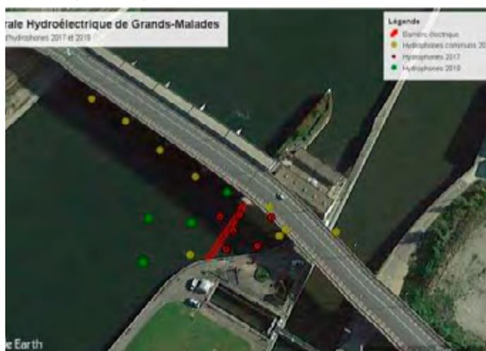
Nevertheless, considering 2017 data and flows < 300 m<sup>3</sup>/s in the Meuse River, for which most of the flow is diverted to the power station, the effectiveness of the barrier drops to 52%. This is due to the fact that at higher flows some of the eels run off through the overflows of the dam.
