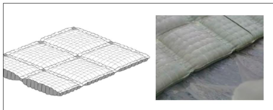
are most often found in use on river banks with susceptible and uncertain substrate. The length of the spacers ranges from 8 to 56 cm, hence the average thickness of the mat can be from 10 to 45 cm. On canals, these mats are used on the excavated sections, i.e. when there may be groundwater inflow into the canal.
