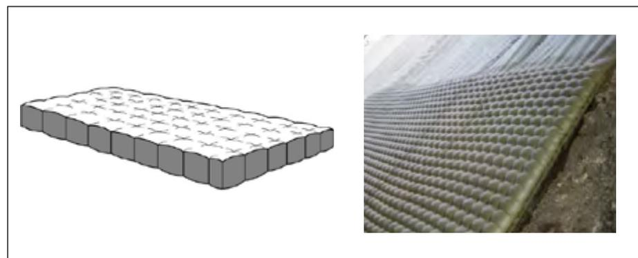
Fig. 3. Incomat® Flex (left) schematic sketch with cross section, (right) view of mattress after concrete filling, photo: Huesker.
