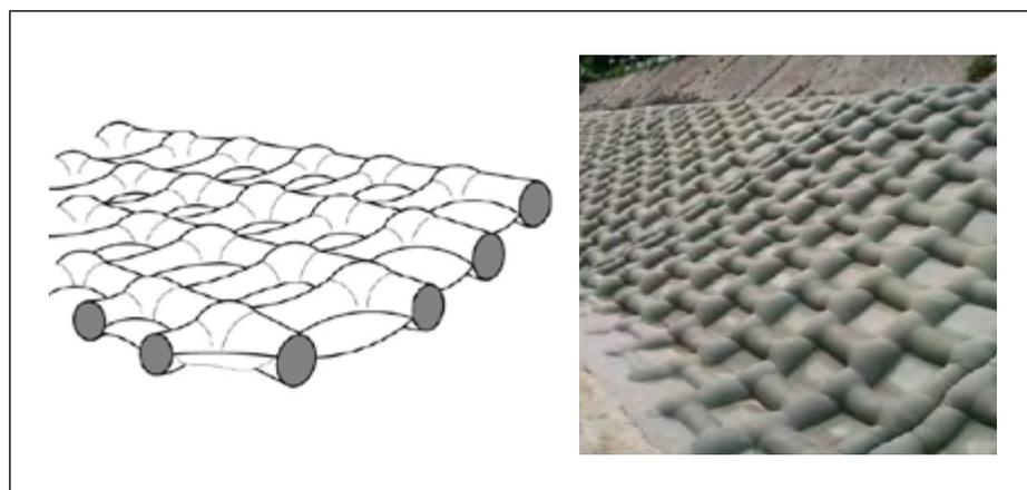
Fig. 6. Canal de la Gentile, (left) mats laid and top anchored, (right) sequential concrete filling, Incomat® Standard 1999–2000, photo: Huesker.
